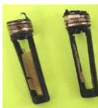
The missing bits of mesh of the damaged filter baskets are now inside the injector and as the injector has a seat with micron tolerances, there is no way these bits of mesh will pass through the injector.
