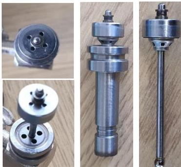
This now creates a problem inside the injector where bits of broken nylon are restricting the injectors' operating functions, for example the fuel delivery quantity, the travel of the pintle and the possibility of these particles causing the injector to leak or cause the injector to stick open and cause hydraulic lock.
