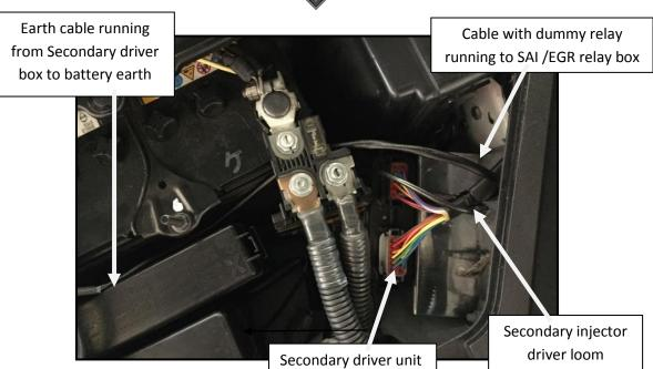
Run the driver harness along the back of the bulkhead/firewall until you reach the centre of
