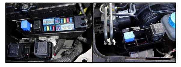
• Connect the main driver harness to the driver box. The plugs are different and will only fit one way round; ensure they are fully engaged.
