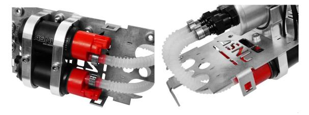
6. Fit zip tie to the pre-filter plate, and pass round the central retaining bolt on the front pump mount
