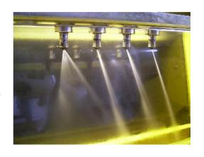
**Fact:** If you had 6 injectors and 6 different deliveries, with the help of the EMS the engine would run correctly. With 6 different spray patterns and 6 correct deliveries, the engine would run badly.
