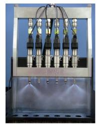
ASNU's engineers then looked at the ability of testing the injectors at systems pressure. Producing a system that could safely show the operation of the injector at high pressure was not a problem, but seeing exactly what the injector was physically doing at high pressure when compared to low pressure testing made the high pressure function more of a disadvantage than a benefit.
