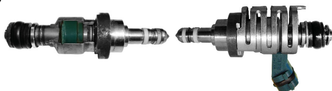
Broken off connector plug due to incorrect removal (should look like the injector to the right)
